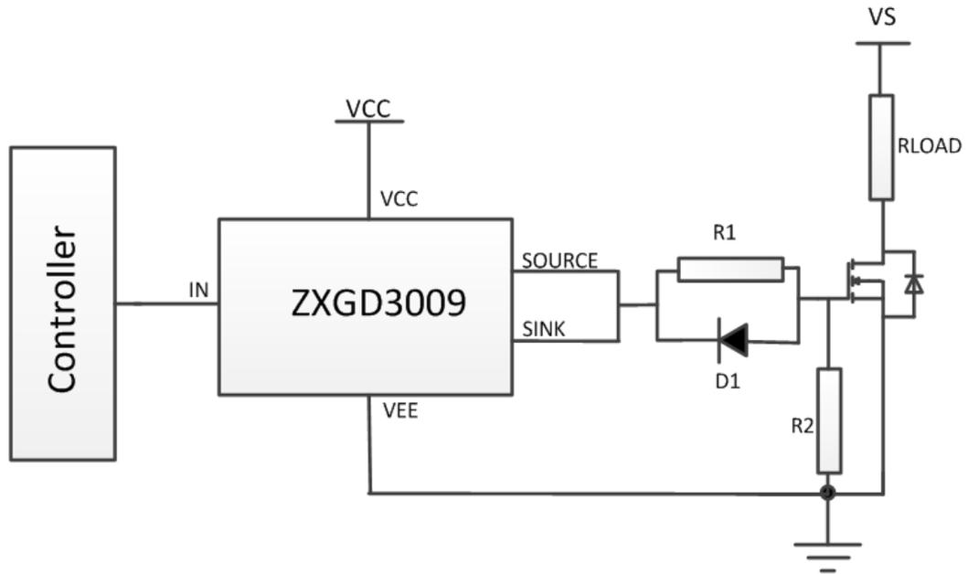
R1, D1 combination can be used for variable turn on and turn off times.
