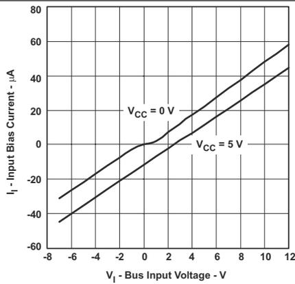
Figure 1. Bus Input Current versus Bus Input Voltage
