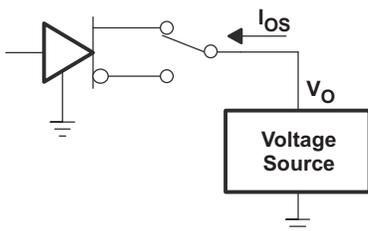
Figure 14. Driver Short-Circuit
