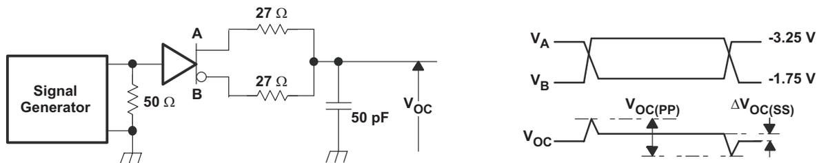
**Figure 10. Driver  $V_{OC}$  Test Circuit and Waveforms**
