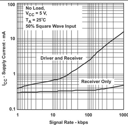
Figure 3. SN65HVD3085E RMS Supply Current versus Signaling Rate
