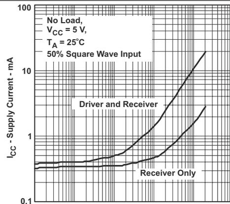
Figure 4. SN65HVD3088E RMS Supply Current versus Signal Rate
