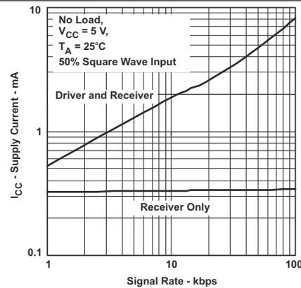
Figure 2. SN65HVD3082E RMS Supply Current versus Signaling Rate
