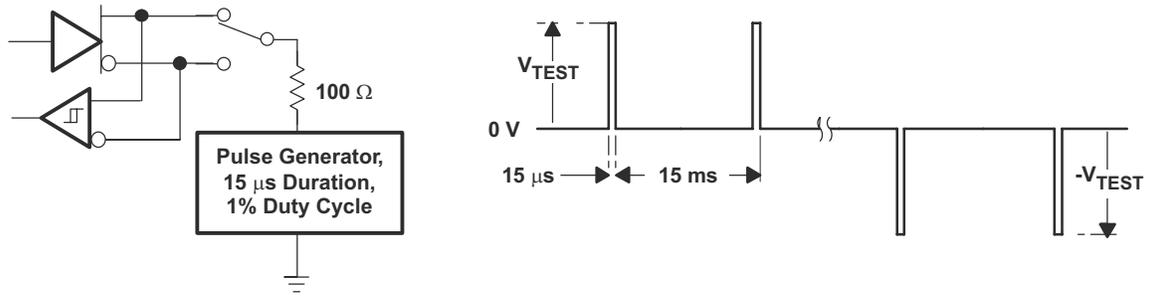
Figure 20. Test Circuit and Waveforms, Transient Overvoltage Test
