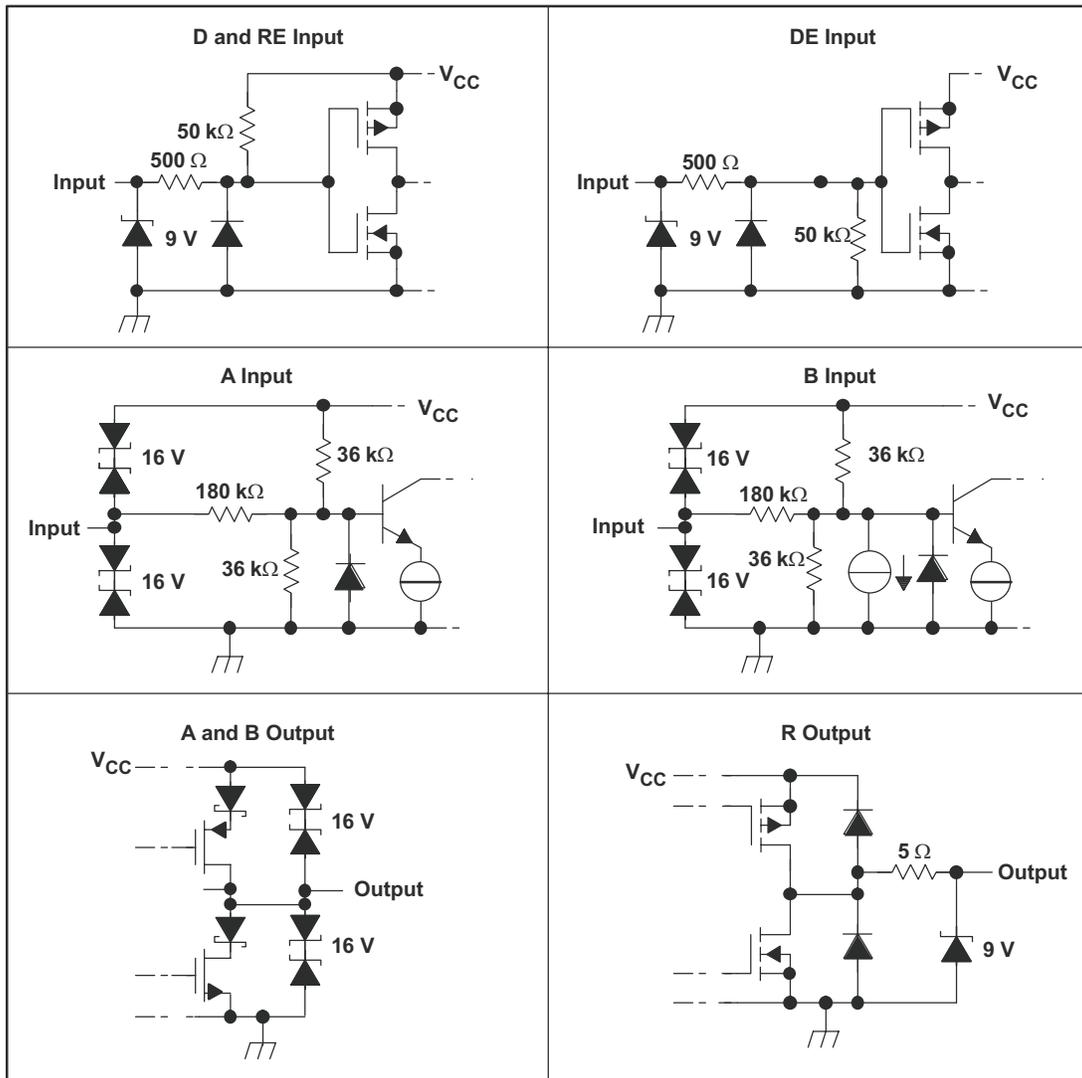
Figure 21. Equivalent Input and Output Schematic Diagrams
