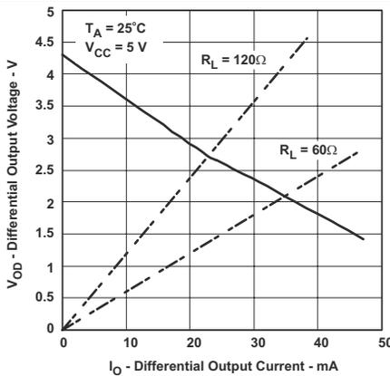
Figure 5. Driver Differential Output Voltage versus Driver Output Current
