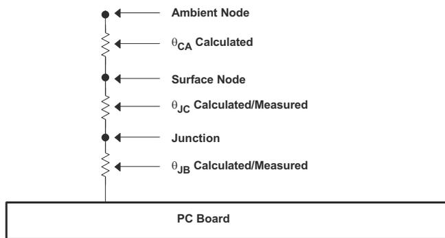
Figure 27. Thermal Resistance
