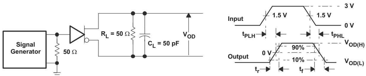
**Figure 11. Driver Switching Test Circuit and Waveforms**
