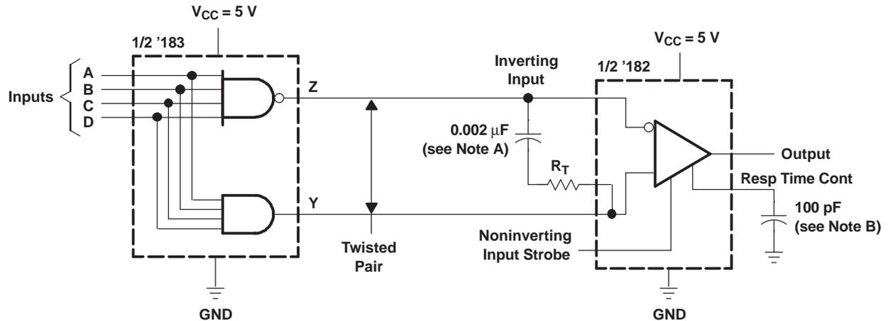
NOTES: A. When the inputs are open circuited, the output is high. A capacitor may be used for dc isolation of the line-terminating resistor. At the frequency of operation, the impedance of the capacitor should be relatively small.
