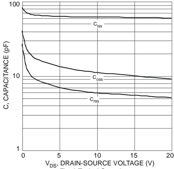
Fig. 9 Typical Capacitance
