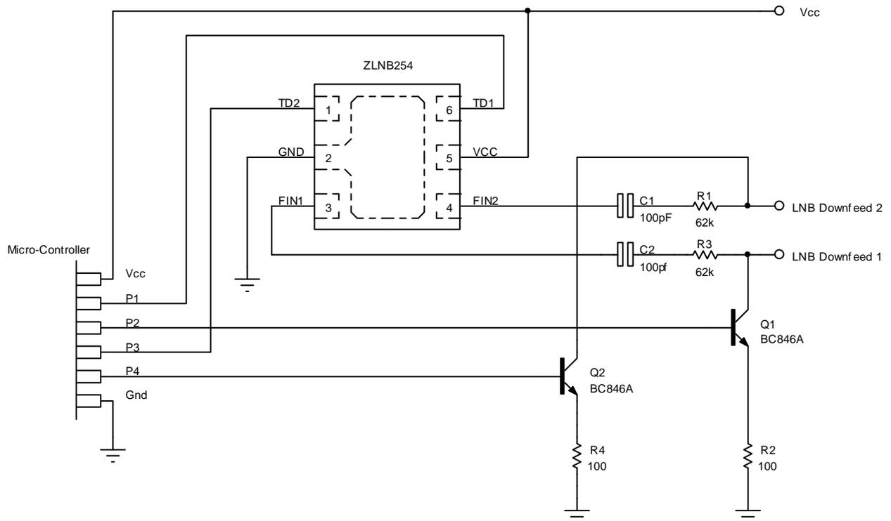
The above circuit shows the additional components that will be used in a typical ZLNB254 application operating at a Vcc of 5V and detecting 22kHz tones/tone bursts. The transistors Q1 and Q2 are not required for the ZLNB254 operation, they demonstrate how a DiSEqC 2.X (2 way communication) could be achieved.
