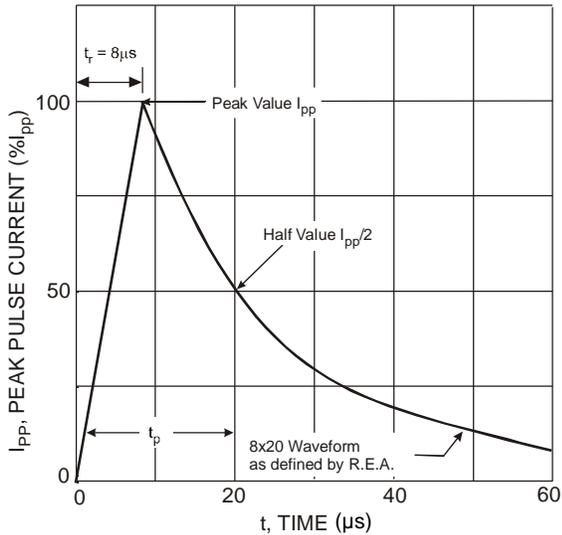
Figure 3 Pulse Waveform
