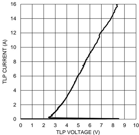
Figure 5 TLP Curve (t<sub>p</sub> = 100ns)
