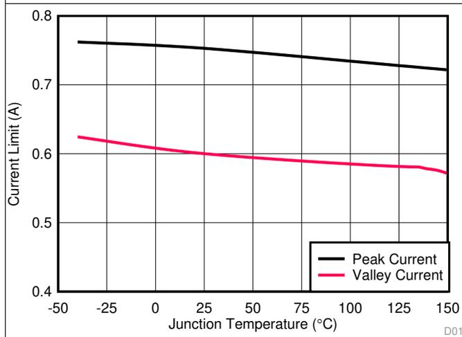
图 9. Peak and Valley Current Limit versus Temperature
