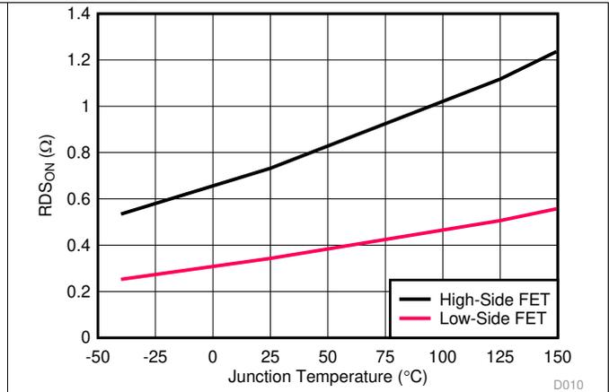
图 8. MOSFETs On-State Resistance versus Temperature
