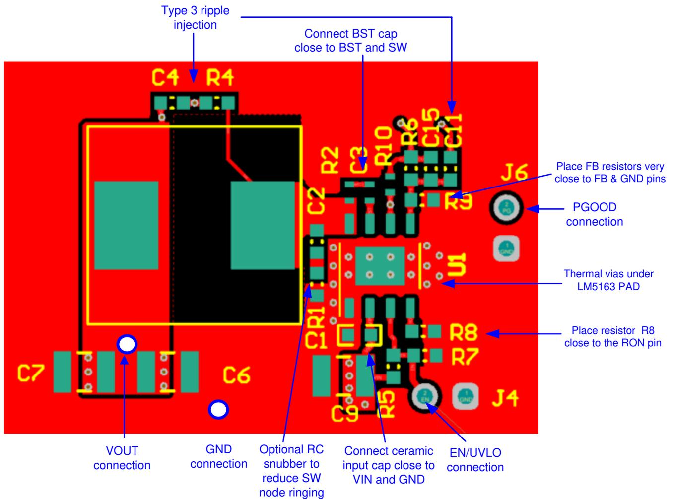
图 30. LM5163 Single-Sided PCB Layout Example
