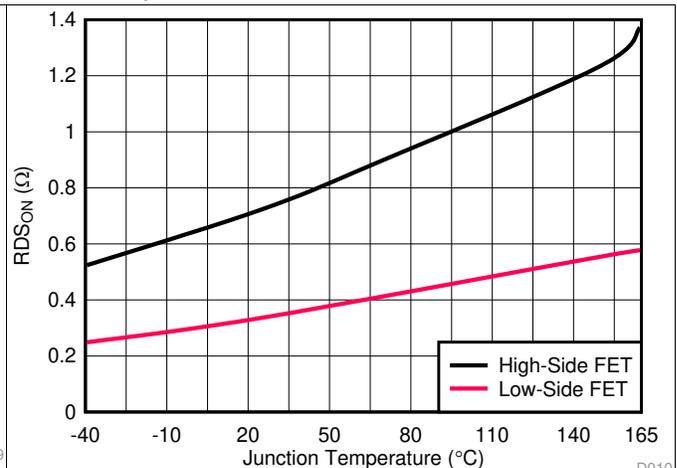
图 8. MOSFETs On-State Resistance versus Temperature
