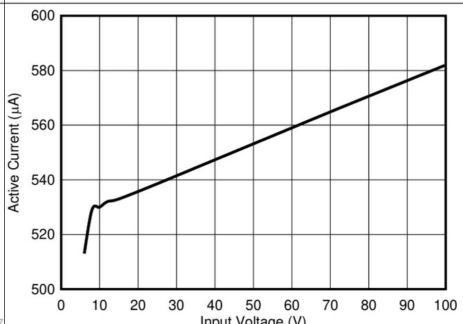
图 6.  $V_{IN}$  Active Current versus Input Voltage
