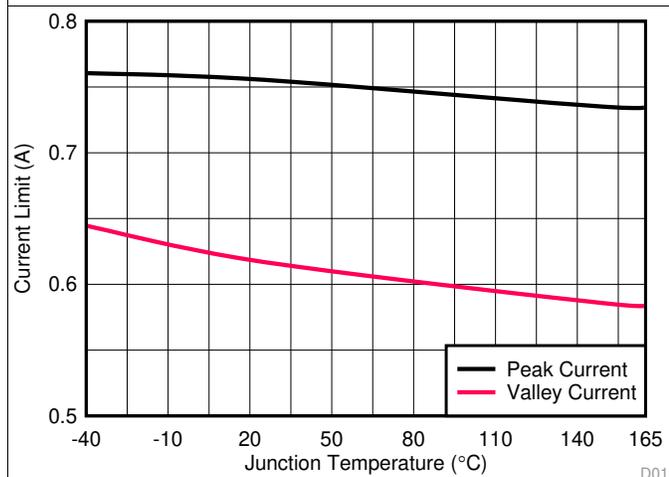
图 9. Peak and Valley Current Limit versus Temperature
