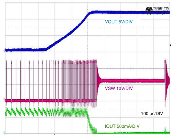
$V_{IN} = 24\text{ V}$  Load = Short to 0 A
