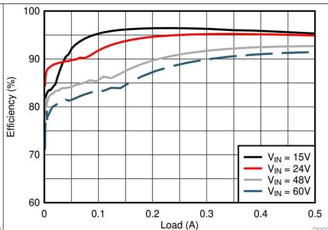
图 2. Conversion Efficiency (Linear Scale)
