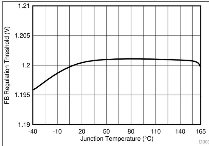
图 7. Feedback Comparator Threshold versus Temperature
