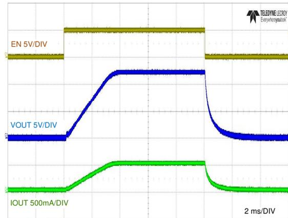
$V_{IN} = 24\text{ V}$   $I_{OUT} = 0.5\text{ A (Resistive)}$
