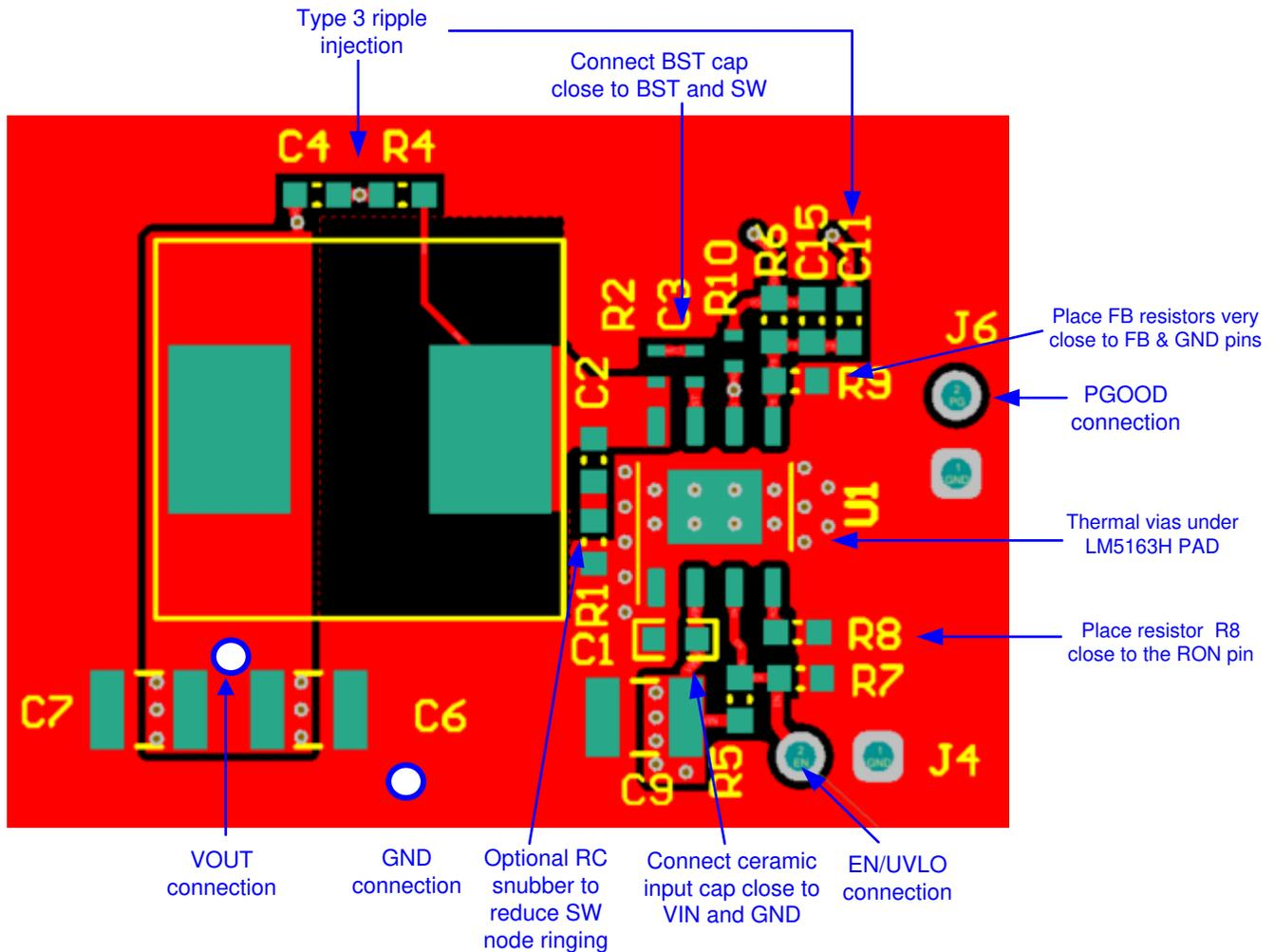
图 30. LM5163H-Q1 Single-Sided PCB Layout Example
