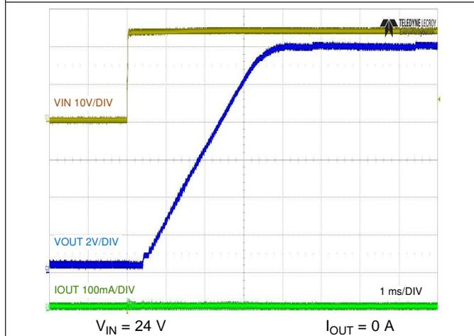
图 17. No-Load Start-up with VIN
