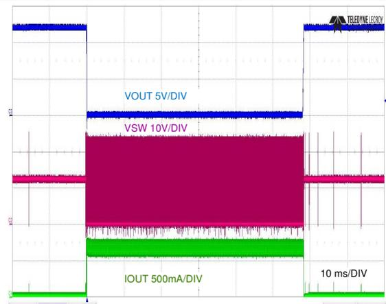
$V_{IN} = 24\text{ V}$  Load = 0 A to Short to 0 A
