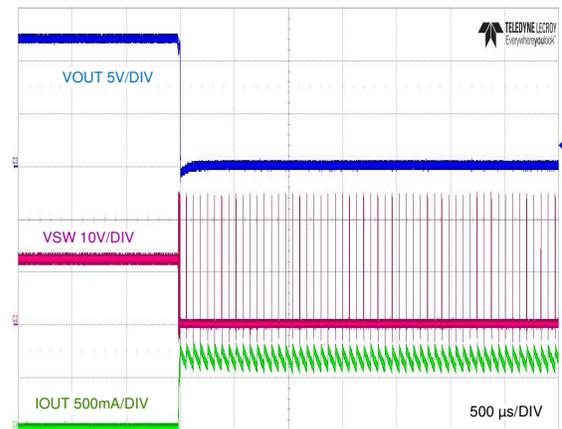
$V_{IN} = 24\text{ V}$  Load = 0 A to Short
