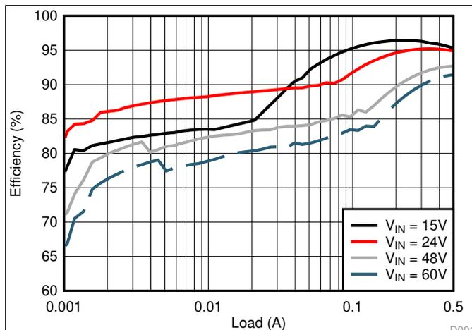
图 1. Conversion Efficiency (Log Scale)
