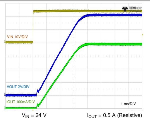
图 18. Full-Load Start-up with VIN
