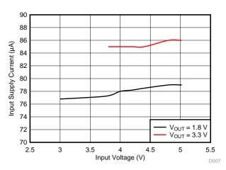
Figure 15. Typical No Load Input Supply Current
