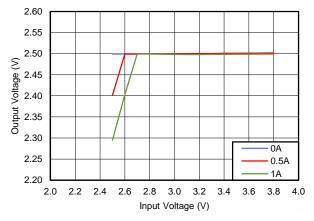
Figure 11. Typical Drop-Out Behavior, V<sub>OUT</sub> = 2.5 V
