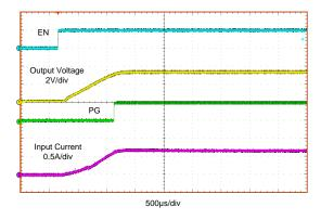
Figure 10. Typical Start-Up Waveforms, V\_{IN} = 5 V, V\_{OUT} = 3.3 V, I\_{OUT} = 1 A
