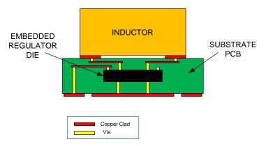
Figure 8. Package Side View Drawing
