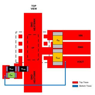
Figure 39. Example PCB Layout
