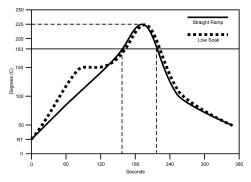
Figure 40. Typical Re-flow Profile Eutectic (63sn/37pb) Solder Paste
