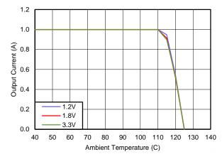
Figure 19. Maximum Output Current Vs. Ambient Temperature, R<sub>0JA</sub> = 44°C/W, V<sub>IN</sub> = 5 V
