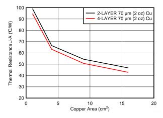
Figure 18.  $R_{\theta JA}$  versus Copper Board Area
