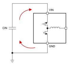
Figure 38. Current Loops With Fast Transient Currents
