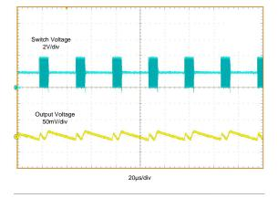
Figure 14. Typical PFM Mode Waveforms: V<sub>IN</sub> = 3.6 V,  $V_{OUT}$  = 1.8 V,  $I_{OUT}$  = 10 mA
