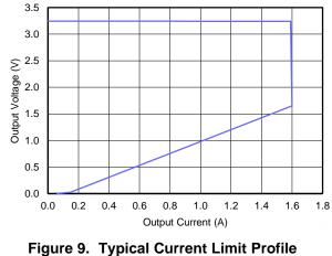
$V_{IN} = 5 V, V_{OUT} = 1.8 V$
