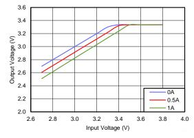
Figure 12. Typical Drop-Out Behavior, V<sub>OUT</sub> = 3.3 V
