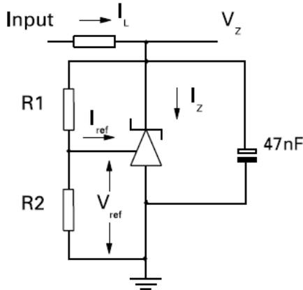
Figure 2. Test Circuit for  $V_Z > V_{REF}$
