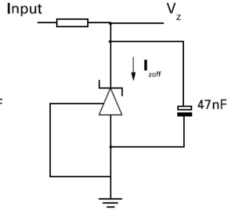
Figure 3. Test Circuit for Off State Current
