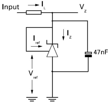
Figure 1. Test Circuit for  $V_Z = V_{REF}$
