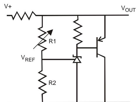
$$V_{OUT} = \left(1 + \frac{R_1}{R_2}\right) V_{REF}$$
