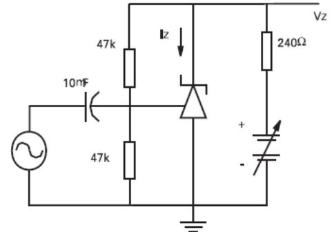
$I_Z = 10\text{mA}$ ,  $T_A = 25^\circ\text{C}$
