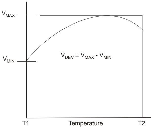
$$V_{ref} \text{ (ppm/}^\circ\text{C)} = \frac{V_{dev} \times 1000000}{V_{ref} (T1 - T2)}$$
