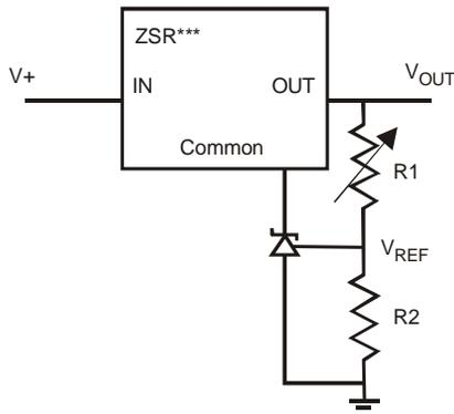
$$V_{OUT(MIN)} = V_{REF} + V_{REG}$$
