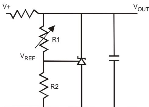
$$V_{OUT} = \left(1 + \frac{R_1}{R_2}\right) V_{REF}$$
