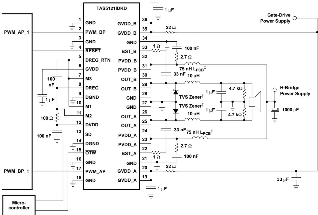
† Voltage suppressor diodes: 1SMA33CAT3
