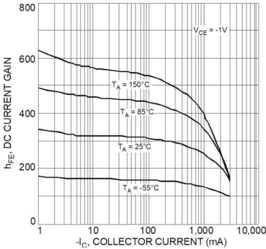
Fig. 5 Typical DC Current Gain vs. Collector Current
