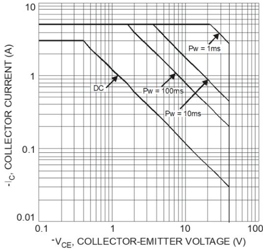
Fig. 3 Typical Collector Current vs. Collector-Emitter Voltage (Note 6)
