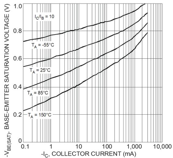
Fig. 8 Typical Base-Emitter Saturation Voltage vs. Collector Current
