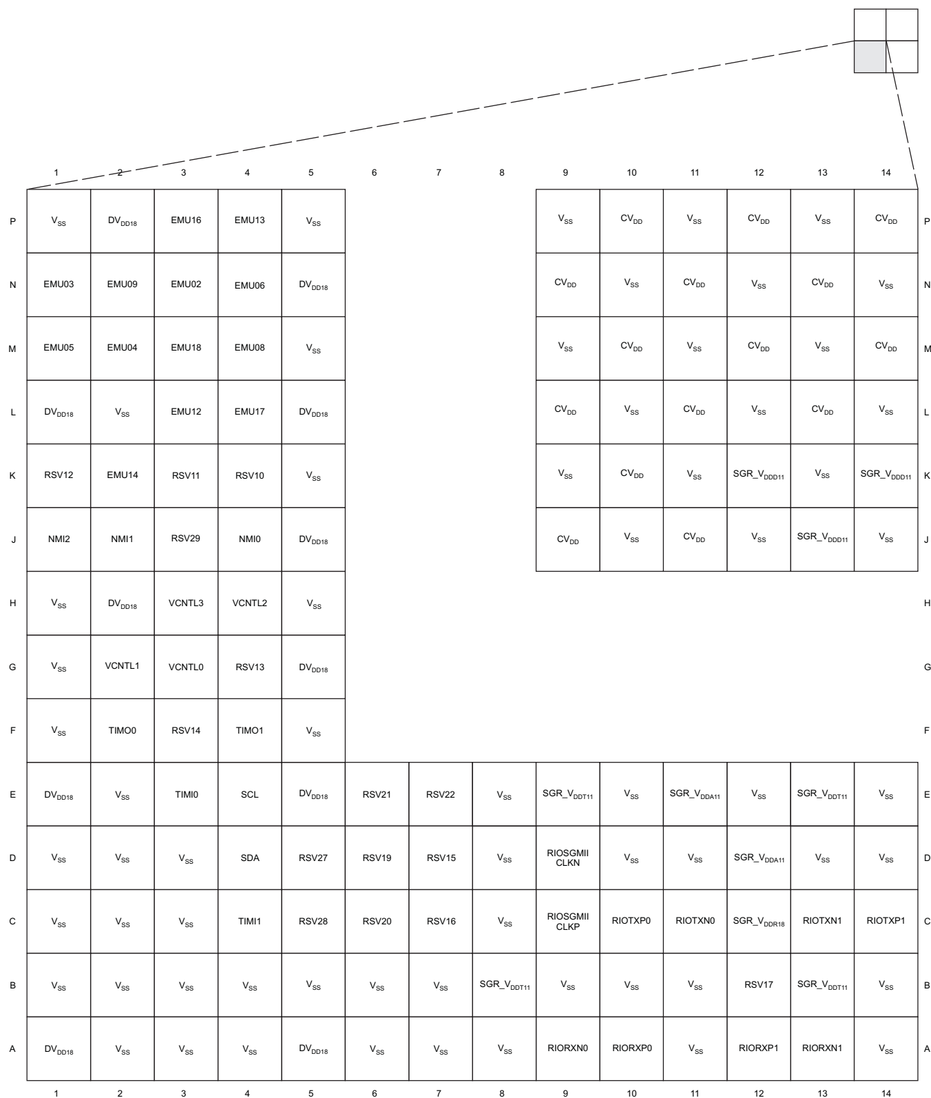
Figure 2-5. C6474 Pin Map (Bottom View) [Quadrant D]
