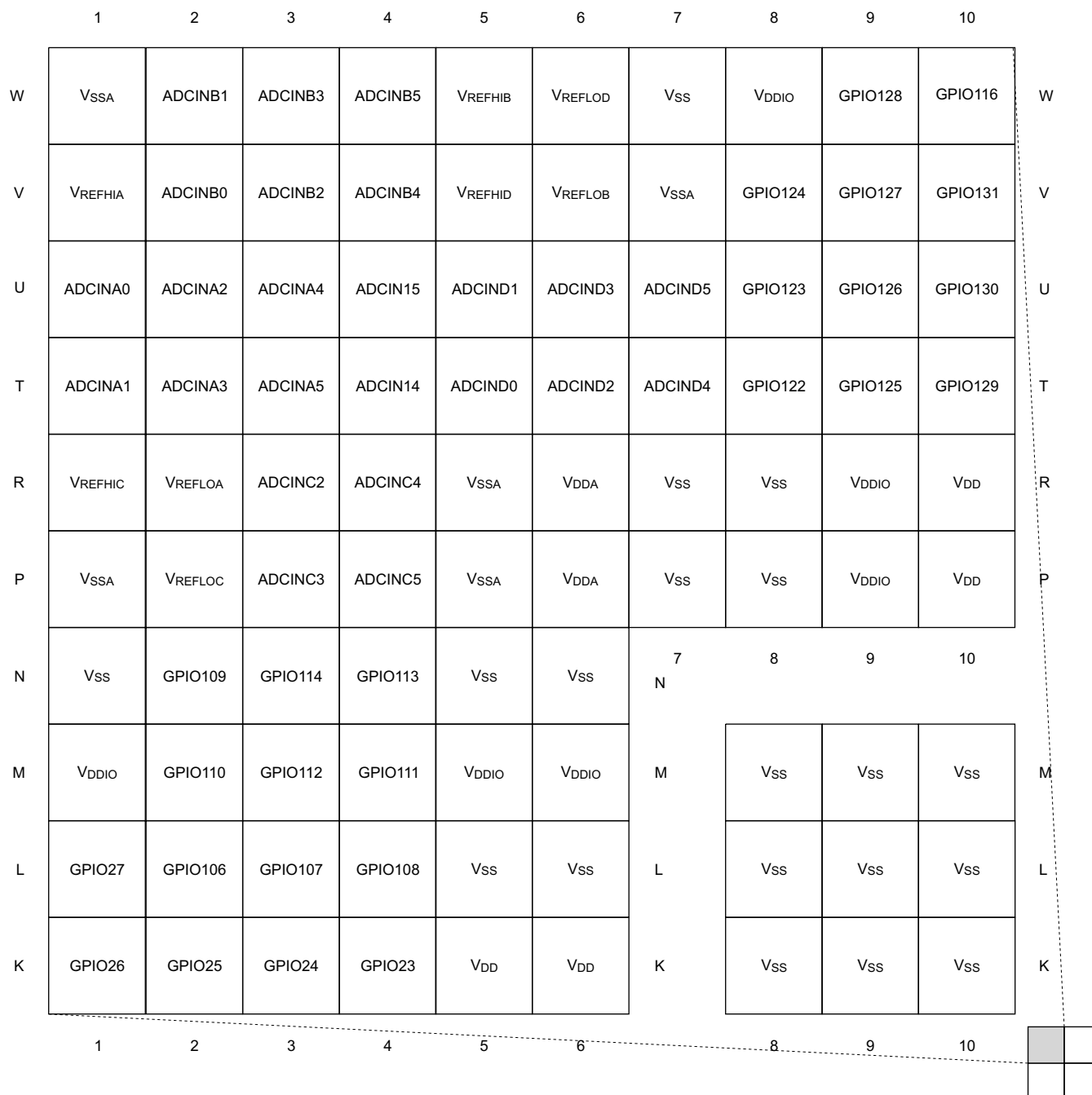
Figure 4-1. 337-Ball ZWT New Fine Pitch Ball Grid Array (Bottom View) – [Quadrant A]
