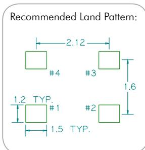
\*Extended high frequency power decoupling is recommended (see test circuit for minimum recommendation). To ensure optimal performance, do not route RF traces beneath the package.
