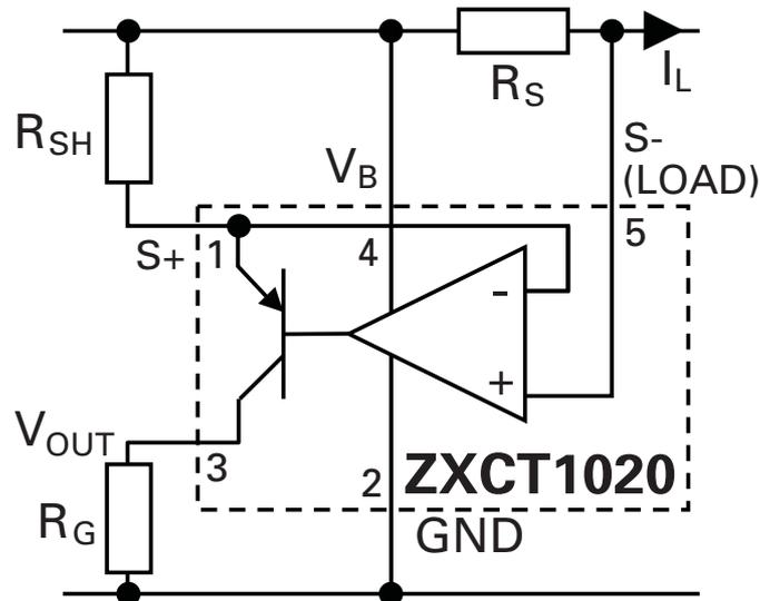
$R_{SH}$  sets the transconductance whereas  $R_G$  set the gain and results in an output voltage defined as:
