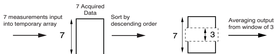
Figure 28. MAV Filter Operation (Patent Pending)
