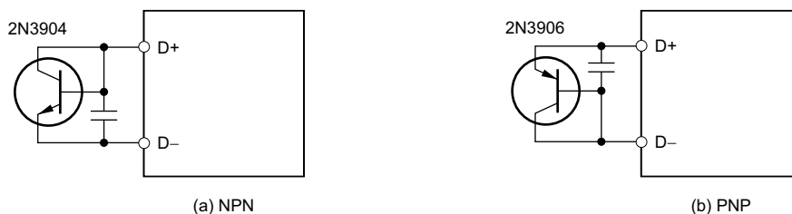
Figure 88. Remote Temperature Sensor Using Transistor
