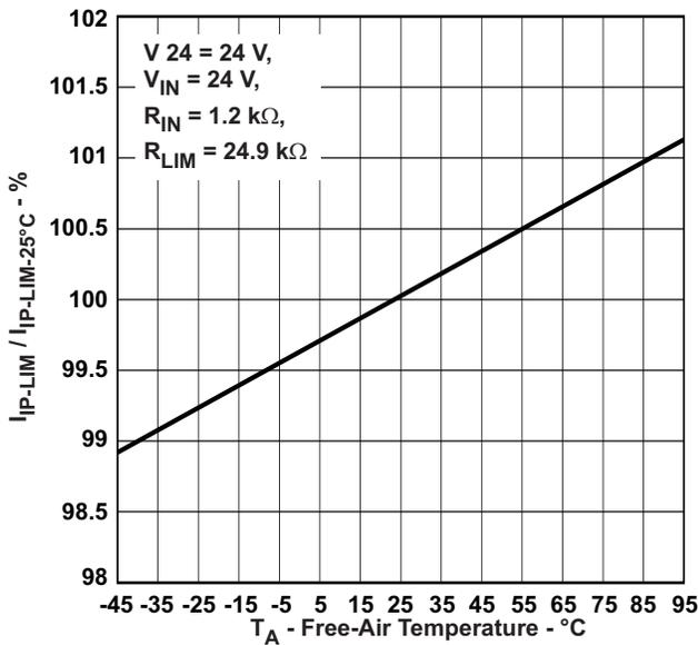
Figure 2. Typical Current Limiter Variation vs Ambient Temperature
