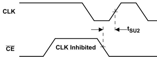
Figure 8. Serial - Shift Clock Inhibit Mode
