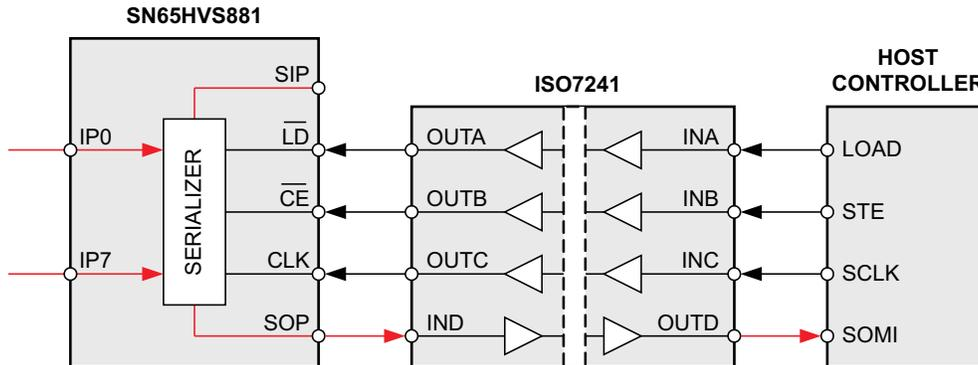
Figure 20. Simple Isolation of the Shift Register Interface
