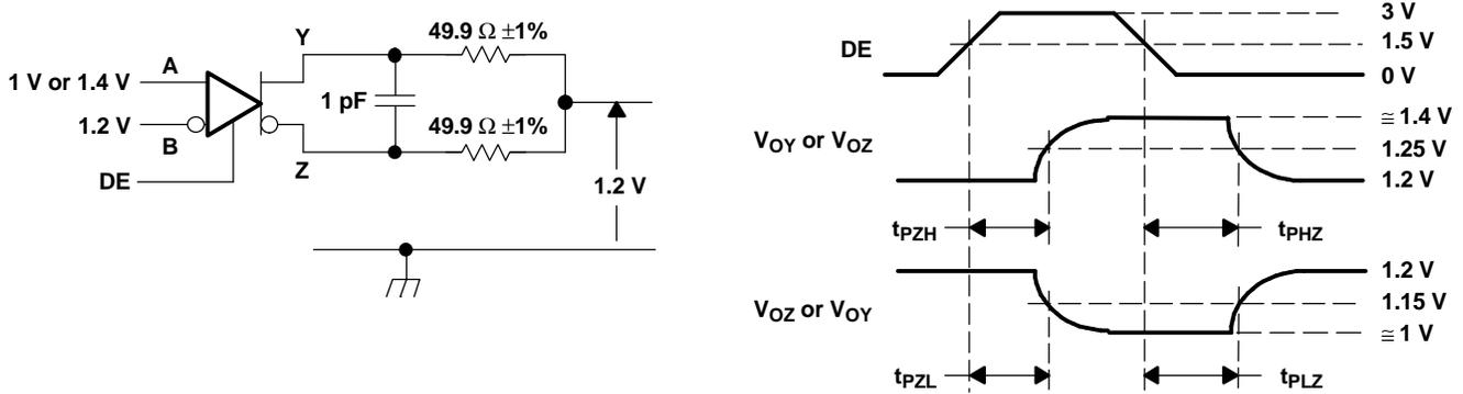
NOTE: All input pulses are supplied by a generator having the following characteristics:  $t_r$  or  $t_f \leq 1$  ns, pulse repetition rate (PRR) = 0.5 Mpps, pulse width =  $500 \pm 10$  ns.  $C_L$  includes instrumentation and fixture capacitance within 0,06 mm of the D.U.T.
