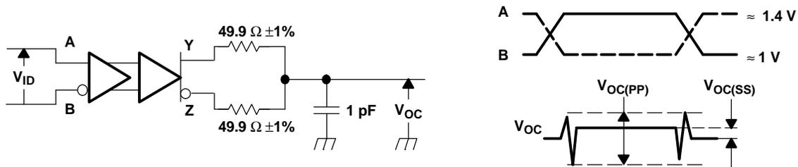
NOTE: All input pulses are supplied by a generator having the following characteristics:  $t_r$  or  $t_f \leq 0.25$  ns, pulse repetition rate (PRR) = 0.5 Mpps, pulse width =  $500 \pm 10$  ns;  $R_L = 100 \Omega$ ;  $C_L$  includes instrumentation and fixture capacitance within 0,06 mm of the D.U.T.; the measurement of  $V_{OC(PP)}$  is made on test equipment with a  $-3$ -dB bandwidth of at least 300 MHz.
