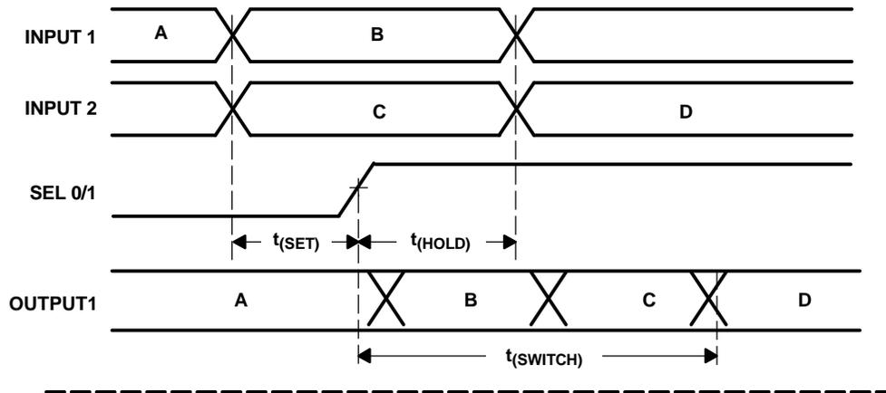
Figure 6. Example Switch, Setup, and Hold Times
