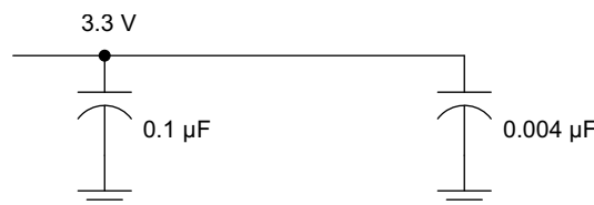
Figure 8-2. Recommended M-LVDS Bypass Capacitor Layout
