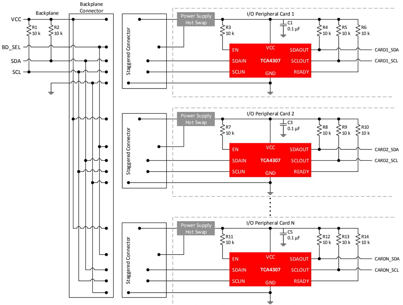
**Figure 9-6. Backplane Application Schematic**
