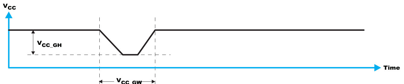
Figure 30. Glitch Width and Glitch Height
