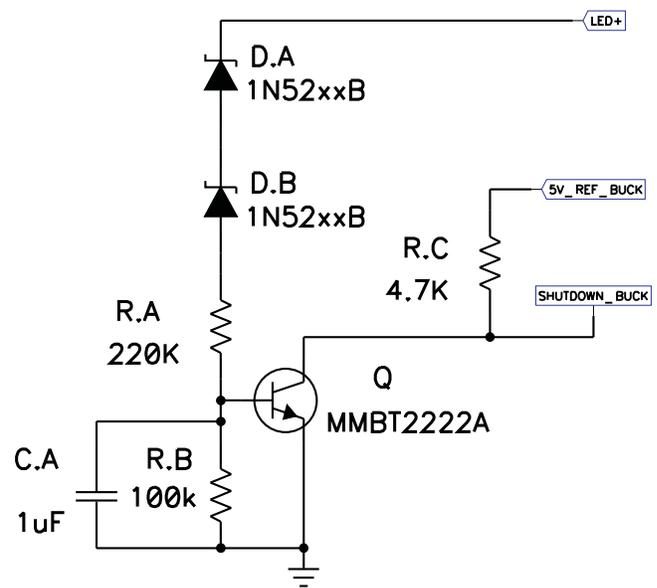
Figure 28. Low-Side Buck UVLO Circuit
