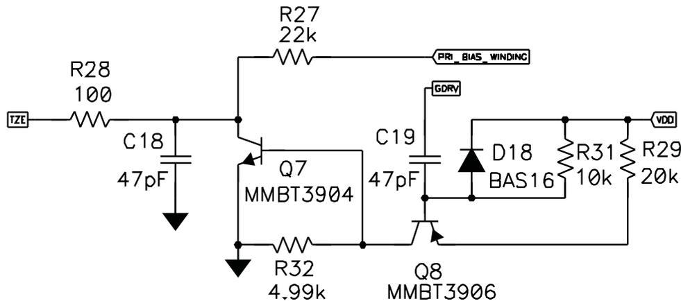
Figure 21. Leading Edge Blanking Circuit on TZE
