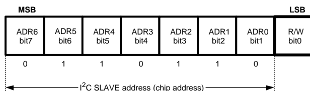
Figure 8. I 2 C Chip Address
