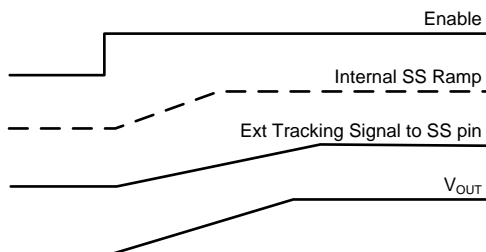
Figure 38. Tracking With Longer Start-up Time Than Tthe Internal Ramp
