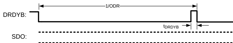
Figure 58. DRDYB Behavior for an ADC_DOUT not Read
