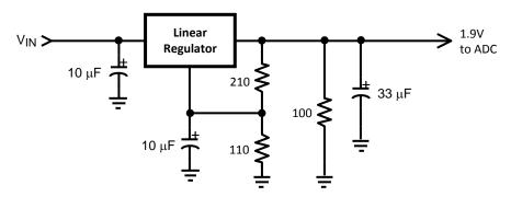
Figure 56. Non-Spiking Power Supply
