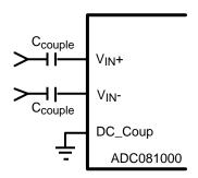
Figure 52. Differential Input Drive
