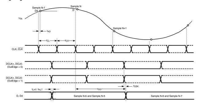
Figure 3. ADC081000 Timing
