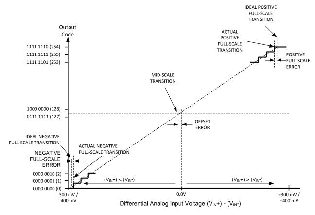
Figure 2. Input / Output Transfer Characteristic
