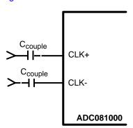
Figure 55. Differential (LVDS) Clock Connection
