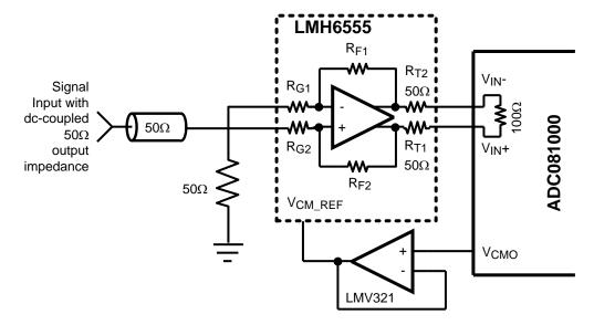
Figure 54. Example of Servoing the Analog Input with V<sub>CMO</sub>
