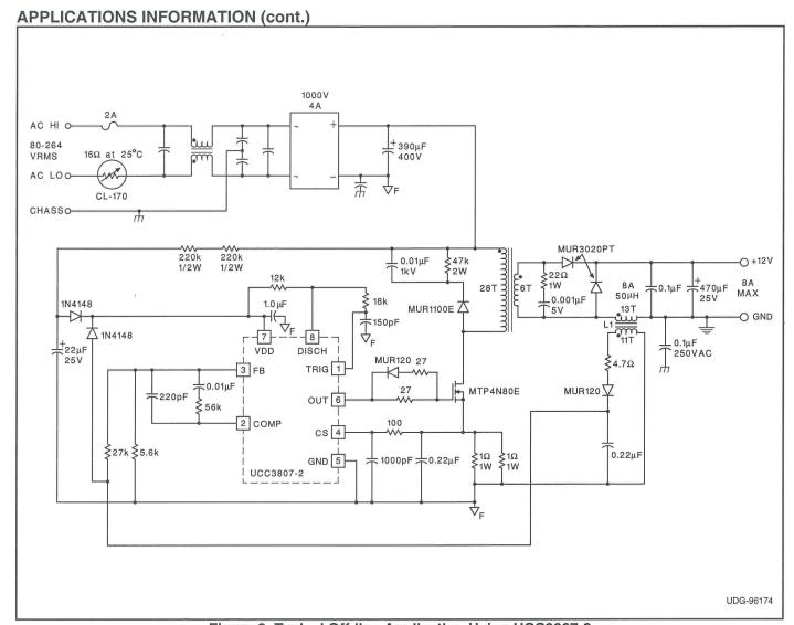
Figure 2. Typical Off-line Application Using UCC3807-2
