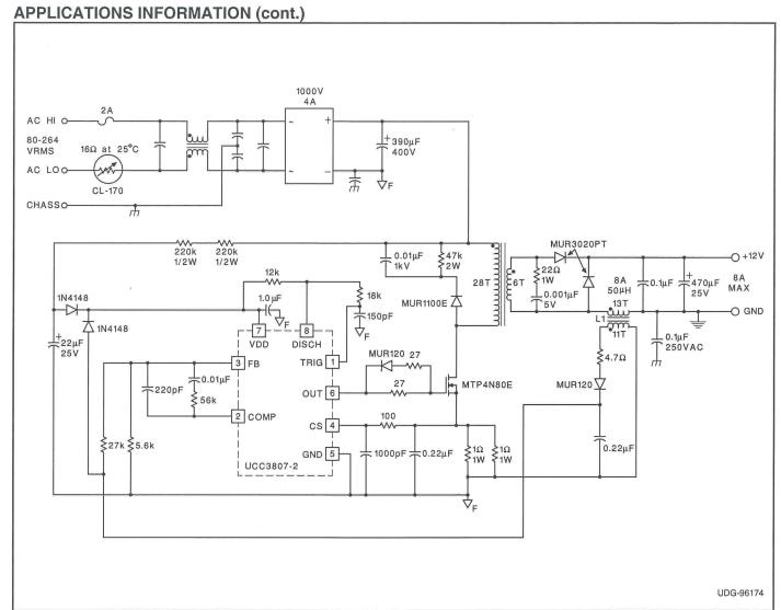
Figure 2. Typical Off-line Application Using UCC3807-2
