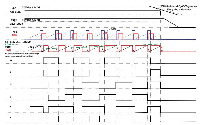
No output delay shown, COMP-to-RAMP offset not included.
