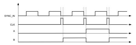
Figure 44. SYNC\_IN (Slave Mode) Timing Diagram
