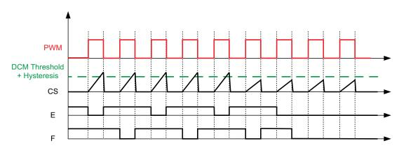
Figure 41. Moving from CCM to DCM Mode
