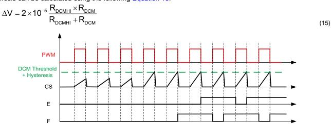
Figure 40. Moving from DCM to CCM Mode
