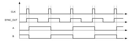
Figure 43. SYNC\_OUT (Master Mode) Timing Diagram
