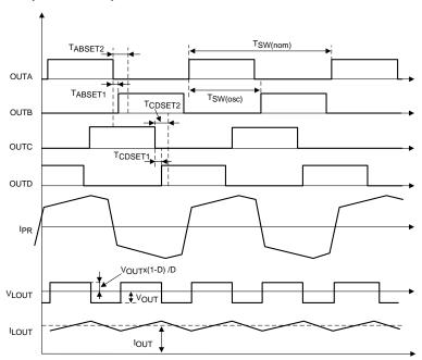
Figure 46. Major Waveforms of Phase-Shifted Converter
