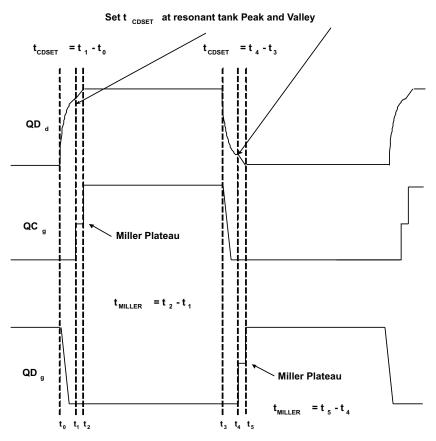
Figure 54. t<sub>CDSET</sub> to Achieve Valley Switching at Light Loads
