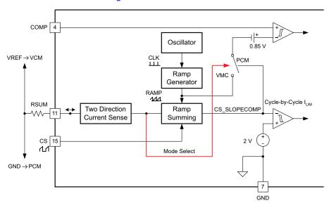
Figure 36. The Operation Logic of Slope Compensation Circuit
