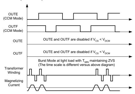
Figure 47. Major Waveforms During Transitions Between Different Operating Modes
