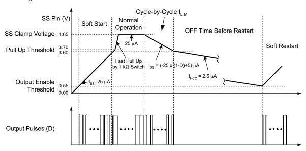
Figure 42. Timing Diagram of Soft-Start Voltage V<sub>SS</sub>
