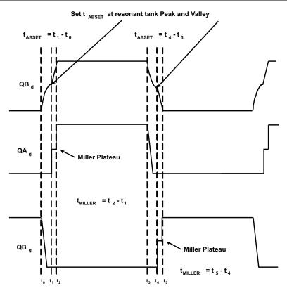
Figure 53. t<sub>ABSET</sub> to Achieve Valley Switching at Light Loads
