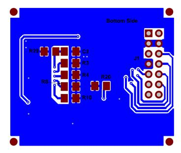
Figure 66. UCC28950 Layout Example (Bottom Side)
