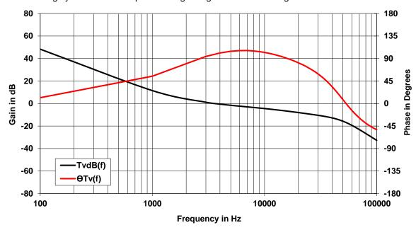
Figure 51. Loop Gain and Phase vs Frequency
