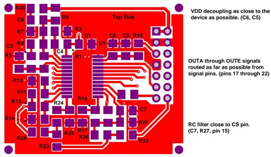
Short tracks at EA+, EA-, COMP, SS/EN, DELAB, DELCD, TMIN, RT, RSUM, DCM, ADELEF, and ADEL pins. (pins 1, 2, 3, 4, 5, 6, 7, 8, 9, 10, 11, 12, 13 and 14)
