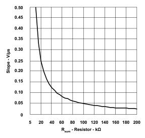
Figure 37. Slope of the Added Ramp Over Resistor R<sub>SUM</sub>
