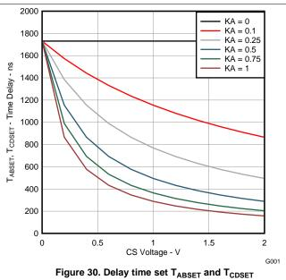
Figure 30. Delay time set  $T_{ABSET}$  and  $T_{CDSET}$  (Over CS voltage variation and selected  $K_A$  for  $R_{AB}$  and  $R_{CD}$  equal 90  $k\Omega$ )
