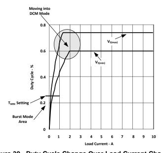
Figure 39. Duty Cycle Change Over Load Current Change
