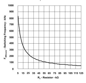
Figure 35. Converter Switching Frequency F<sub>SW(nom)</sub> Over resistor R<sub>T</sub> Value
