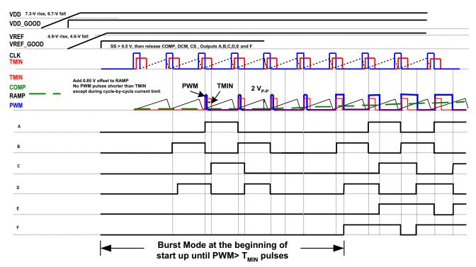
No output delay shown, COMP-to-RAMP offset not included.
