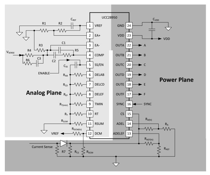
Figure 45. Layout Recommendation for Analog and Power Planes
