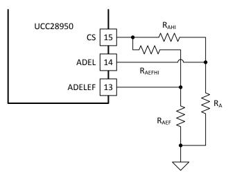
Figure 52. UCC28950 Adaptive Delays
