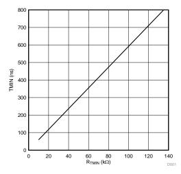
Figure 34. Minimum Time TMIN Over Setting Resistor R<sub>TMIN</sub>
