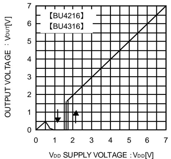
Fig.6 I/O Characteristics
