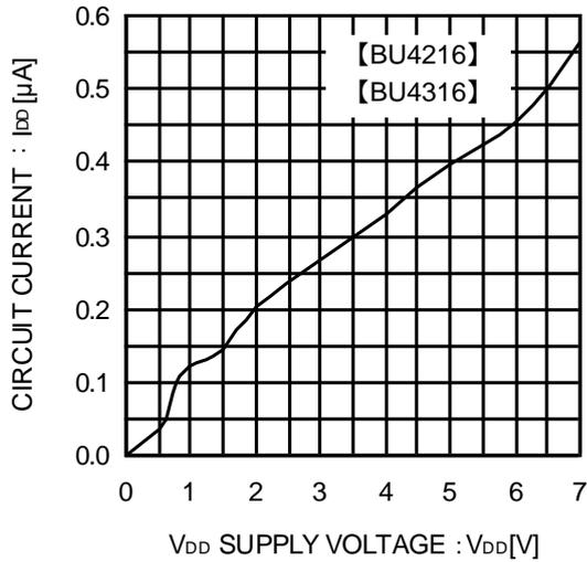
Fig.3 Circuit Current
