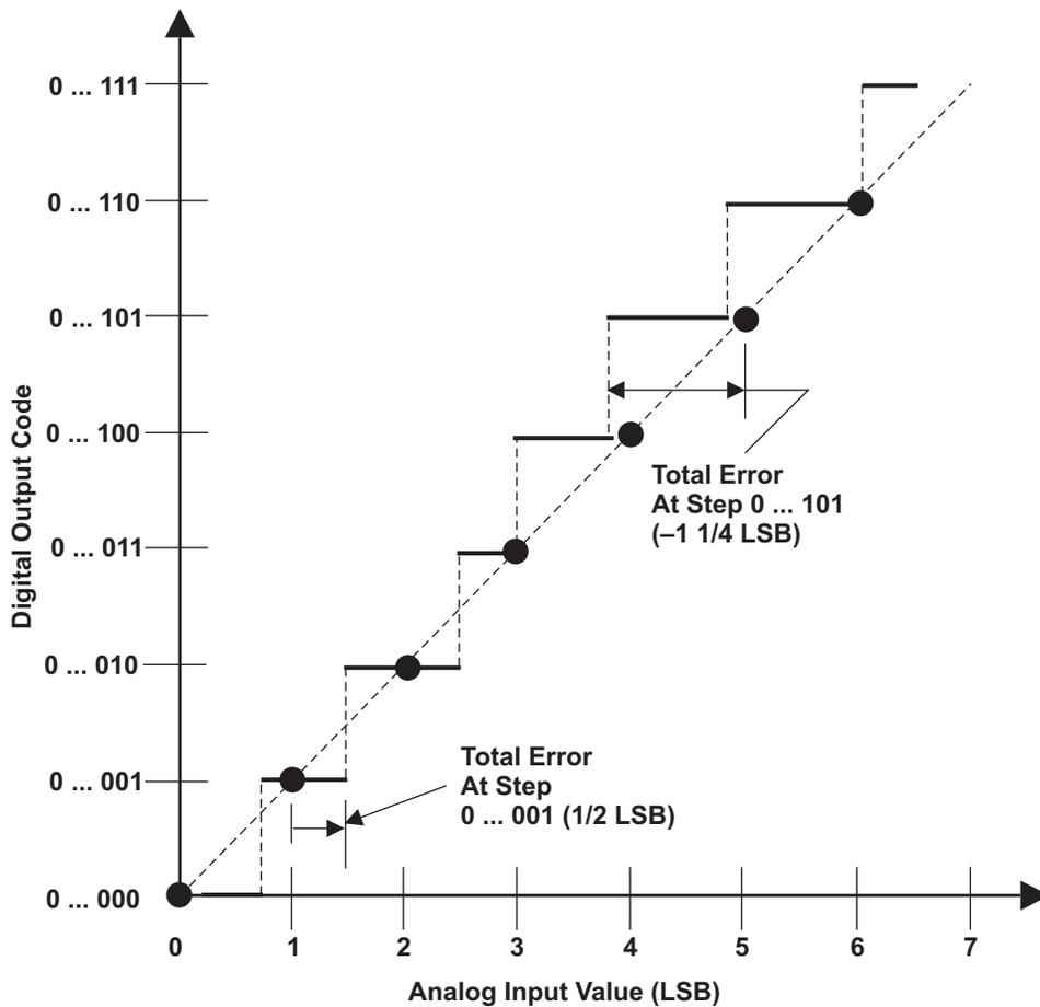
NOTE A:  $1 \text{ LSB} = (\text{AD}_{\text{REFHI}} - \text{AD}_{\text{REFLO}})2^{-12}$
