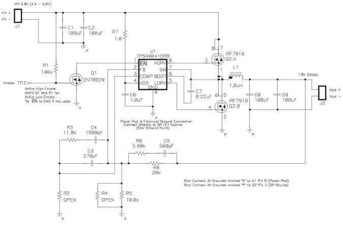
Figure 23. TPS40041 Sample Schematic
