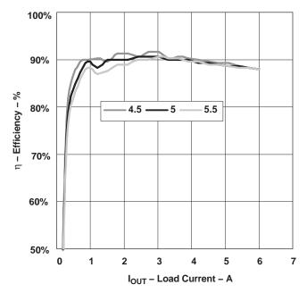
Figure 26. Typical Efficency for 5-V to 1.8-V at 6-A Converter Using TPS40041
