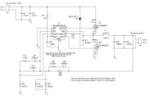
Figure 31. Schematic for 3.3-V to 1.2-V at 10-A Converter Using the TPS40040
