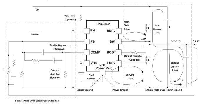
Figure 22. Synchronous BUCK Power Stage
