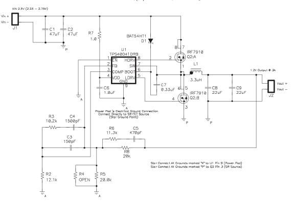
Figure 28. Schematic for 2.5-V to 1.2-V at 3-A Converter Using the TPS40041
