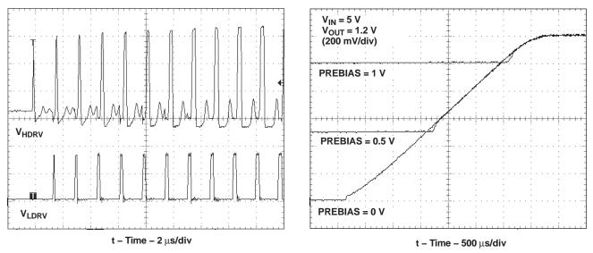
Figure 20. MOSFET Drivers at Beginning of Soft Start
