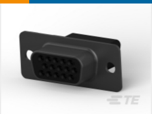
TE 产品编号1658690-1 D-Sub Crimp Recpt Signal 15 Posn, Socket Size 22, Shell Size 1
