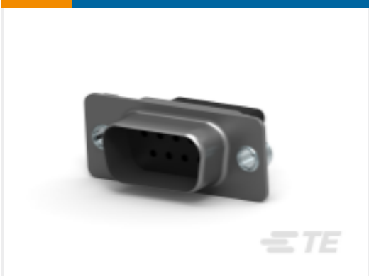
TE 产品编号205204-4 D-Sub Crimp: Plug, Signal, 9 Posn, Pin Size 20, Shell Size 1
