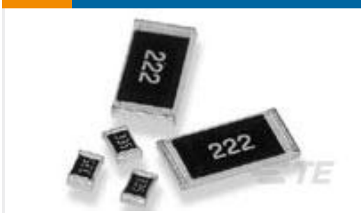
TE 产品编号1-2176177-7 CRGH0603 1% 3K3 0.2W
