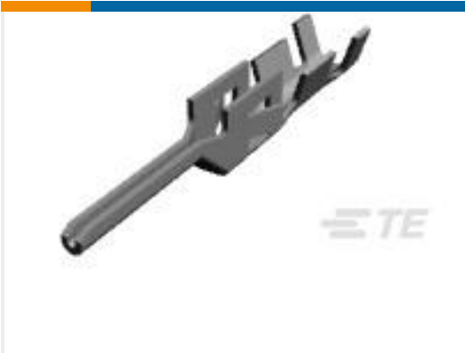
TE 产品编号1-794612-0 PIN CONT 20-24 TIN PLATE L/P
