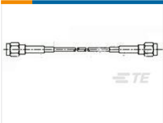
TE 产品编号1337808-1 50 OHM COAX SMA STR PLUG STR P
