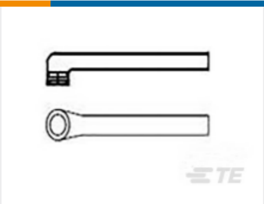
TE 产品编号462378-000 Low Profile Heat Shrink Boots: Poly Mold, Lipped, Right Angle
