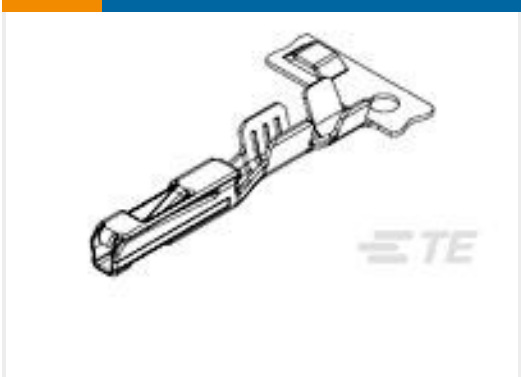
TE 产品编号1326028-2 0.64MM FEMALE CONTACT,AU, 22AWG
