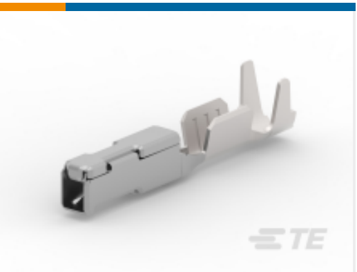
TE 产品编号1456968-3 CONTACT,FEMALE, 0.64, 20 TO 22 AWG, AG
