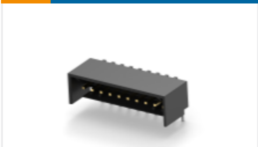
TE 产品编号2-644489-6 Polyester Right Angle PCB Header: 2.54mm, Shrouded, With Mating Alignment
