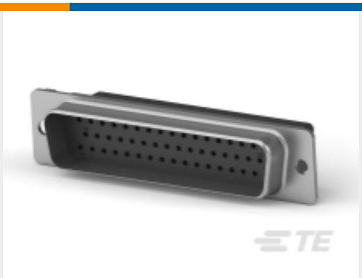
TE 产品编号1658641-2 D-Sub Crimp: Plug, Signal, 50 Posn, Pin Size 20, Shell Size 5
