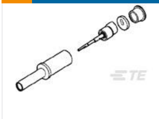
TE 产品编号1757624-1 SZ 8 COAX PIN, RG142, HEX CRIMP
