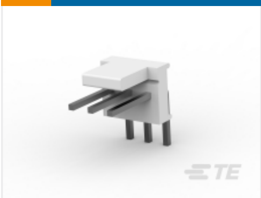
TE 产品编号3-641214-8 Polyester Right Angle PCB Header: 2.54mm, Wire-to-Board, MTA 100
