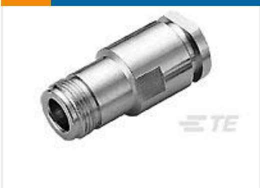
TE 产品编号1-1337406-0 N Str Jk PS 50Ohm Silver Pltd PSF 1 /4M,
