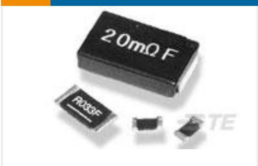
TE 产品编号1-2176155-7 TLM 0805 0.25W R013 1% 100PPM 5K RL
