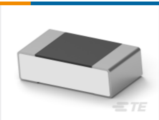
TE 产品编号2-2176371-2 RQ 0603 7K68 0.1% 10PPM 5K RL
