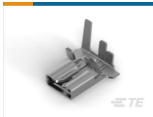
TE 产品编号 2238171-3 250 FASTON,FLAG,REC.,22-12 AWG, TPBR
