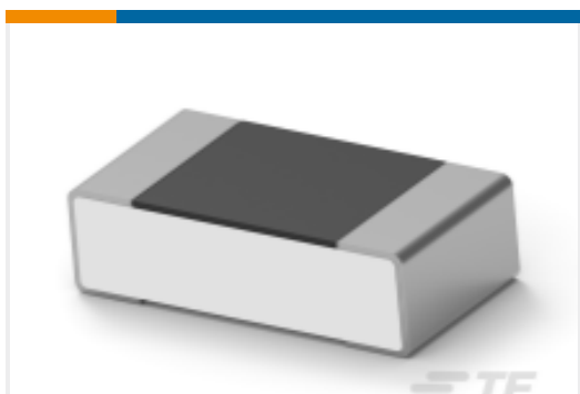
TE 产品编号2-2176371-2 RQ 0603 7K68 0.1% 10PPM 5K RL
